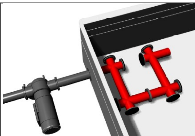
Fig. 7 - Internal tank installation for UltraLED Water 2000/2 System
